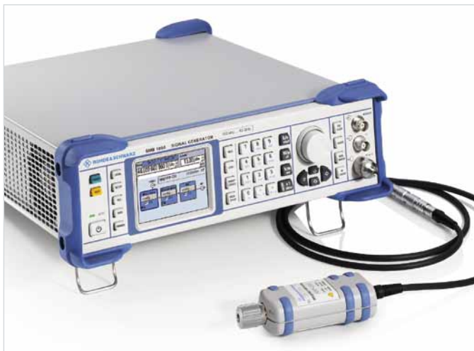
FIG 1 The R&S®SMB100A with the R&S®NRP-Z85 power sensor (connected using the R&S®NRP-Z4 USB adapter cable) for direct level measurement and output to the generator display.
