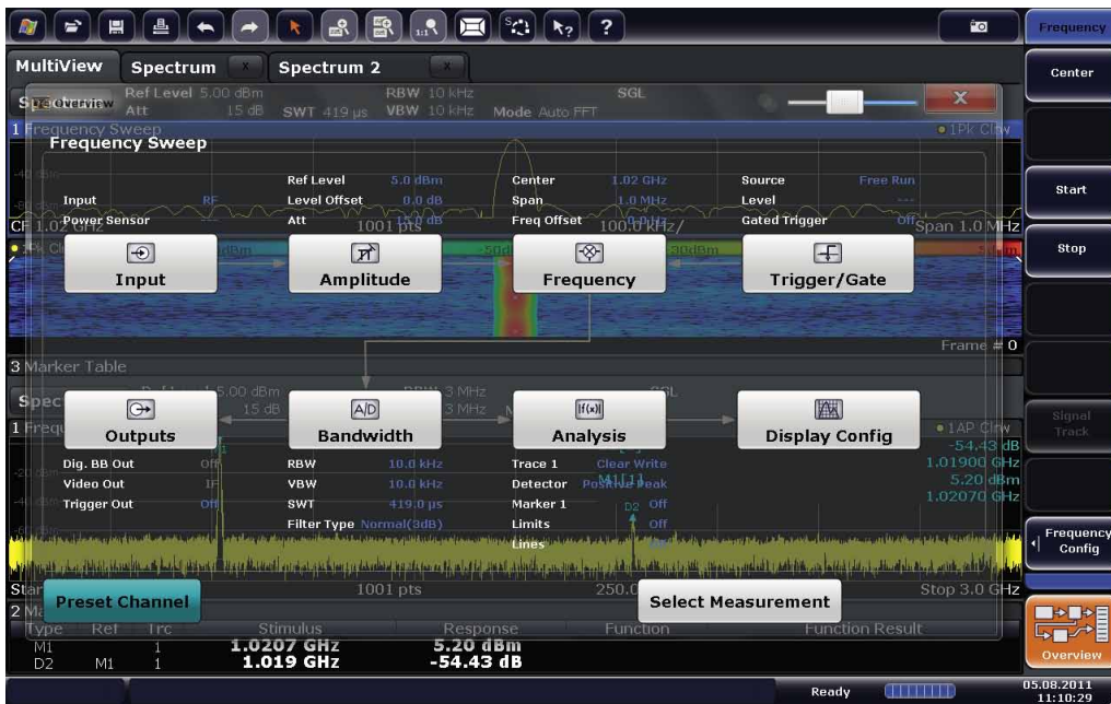
FIG 2 The block diagrams showing the signal flow and the dialog windows for test configuration are transparent, so results remain visible. Any changes in results due to modified settings can be viewed immediately.
