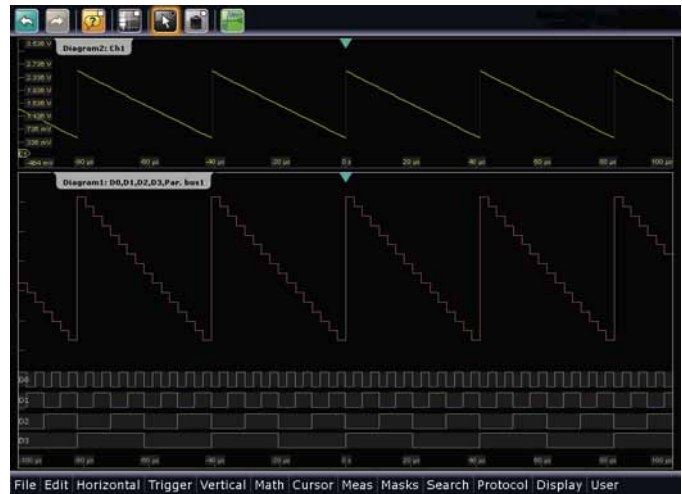
FIG 4 Different presentations of a parallel bus signal as the input signal of an A/D converter (top), as binary signals at the output and as analog waveforms (bottom).
