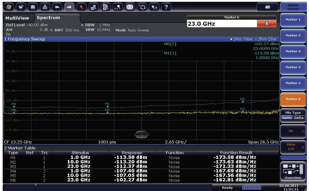
FIG 7 Displayed average noise level (DANL) with preamplifier and noise cancellation switched on.
