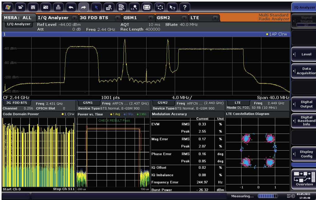
FIG 4 The R&S®FSW's multi-standard radio analyzer measures and displays signals to different standards and at different frequencies in parallel. This example shows four different mobile radio signals: one WCDMA signal, two GSM signals and one LTE signal (from left).
